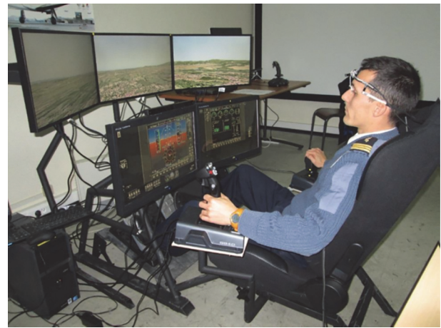
Figure 1. An Air Force Captain engaged in the experiment using the experimental flight simulator. The head-mounted eye tracker is visible.
